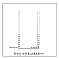
source placed at the actual base of the tower. To make a NEC model of a broadcast tower work, it is thus necessary to use a greater number of segments, which will result in smaller segments. The FCC rules require that base calculations must be made for a reference point at ground level or within one electrical degree elevation of the actual feed point. With the one degree restriction, a segment length of no more than two degrees must thus be used for NEC models.
