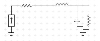
The current source is on the left, and the resistor on the right represents the complex impedance of the tower as modeled.
