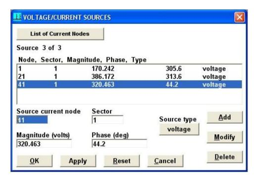
Now we have to re-run the model with the new sources. Later versions of MBPro will bring up a window after the array synthesis has run reminding you of this. Press F5, make sure the õCurrents admittance coupling...ö box is checked and click Ok. You will be prompted for a file save. Change the name to reflect that this run has the correct DA source voltages and phases and save.
