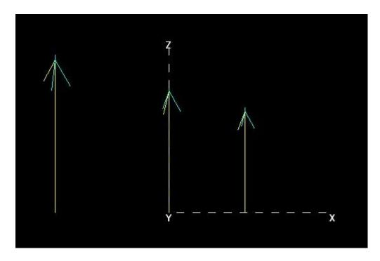
In the model calibration process, the top loading wire length and diameter should remain the same as the effective tower height is being varied.
