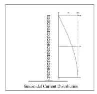
Conventional methods of directional antenna analysis not only assumed sinusoidal current distribution for each tower, but they also required uniform, current distribution for elements in an array. Also, the tower currents used in the calculations were not directly responsible for the far fields for each tower.
