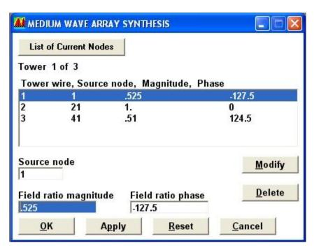
Click Ok. Press F5 to run the model, making sure õCurrents admittance couplingí öis checked. When the Display options screen opens, click array synthesis, type 2200 in the Input power (watts) and click Text. A WordPad document will then open and display the array synthesis, which should look like this:
