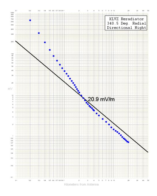
Note how nicely the IDF settles down below standard pattern beyond 2.5 km or so. Also note how the IDF is well above standard pattern inside 2.5 km. Were a monitor point located within that distance on the radial, it would likely indicate a high value that would bear no relationship to what is really going on along the radial in the far field, where it counts.
