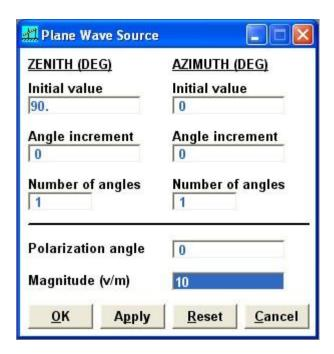
Type ctrl-p and set up a radiation sweep at a single zero zenith and a 72-radial 5-degree increment azimuth.
