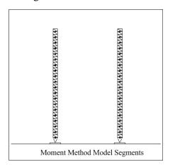
the modeler is careful in his selection of segment length, a close approximation of actual current distribution can be obtained from the model. This has the benefit of predicting base drive impedances much more accurately than any other method. It is not hard to see how knowing the actual current distribution on the tower and the driving point impedances would benefit the engineer designing a phasing and coupling system or tuning up an array.
