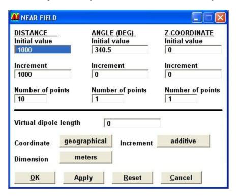
Click Ok. Press F5, be sure ocurrents admittance coupling of and Electric near field are checked and click Ok to run the model. Save the file when prompted.
