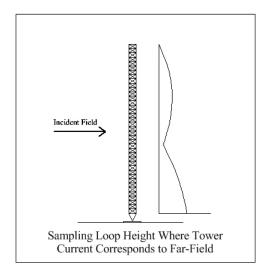
The conventional location for a sample loop is near the base of a short tower, high enough above the base insulator that it is no longer influenced by the base effects but still in the assumed maximum current area of the tower. For taller towers, the conventional location is roughly ¼ wavelength down from the top of the tower, at the current loop (assuming sinusoidal current distribution).
