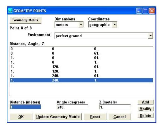
Now we'dl create the wires for the monopole and skirt (ctrl-w). Connect nodes 1 and 2 with a radius of 0.256 and 15 segments for the monopole.
