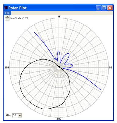
The extent of the pattern distortion is often visible in the radiation pattern, and this is a useful tool to show where the distortion occurs. It is not, however, helpful in determining whether the resultant pattern exceeds the standard pattern.
