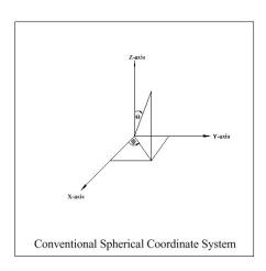
The NEC and MININEC cores use the spherical coordinate system consisting of X, Y and Z axes with units in meters. Azimuth displacement in the X-Y plane is measured from the +X axis and increases in the counter-clockwise direction. The elevation angle is measured from the +Z axis with the zenith being 0 degrees.
