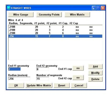
Click Ok to close. Now go to Problem definition | Solution | Near field (or click ctrl-r). We are interested in the null radials first, so let so look at the 340.5 degree radial. Set the coordinate system to geographical and the dimension to meters. Set an initial distance of 1000 meters, an increment of 1000 meters and have it calculate out to 10 km. We only need one angle, 340.5 degrees, and we'll do the calculation at ground level (Z \u00f3 0).
