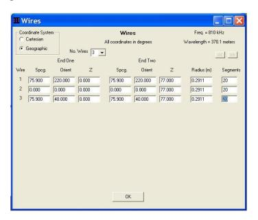
Next, type ctrl-b to enter the directional antenna parameters. Select three towers and enter the array parameters as follows:
