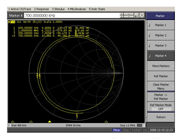
Next, we must determine the characteristic impedance of the line. Again, the FCC rules call for determining the open-circuit resonant frequency closest to the carrier frequency to establish length, and for measuring at frequencies corresponding to odd multiples of 1/8 wavelength immediately above and below that resonant frequency. So we are looking for the frequency that is 1/8 (45 degrees) above and below the resonant frequency. We find those as follows:
