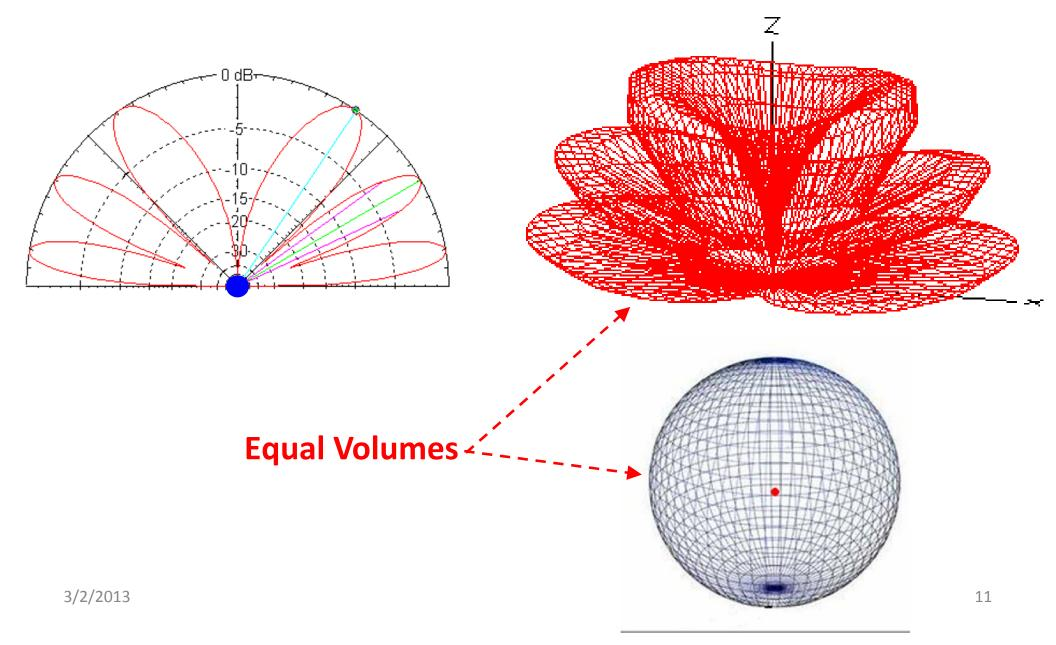
Antenna Directivity vs. Gain vs. Capture Area
