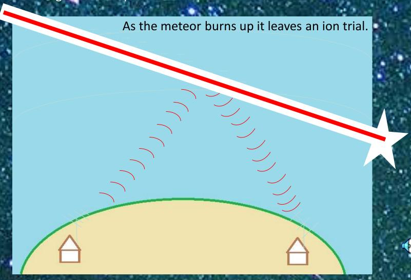
If a radio signal is heading in the direction of the meteor's ion trail it can be reflected back to earth
