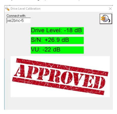
The Ping function show the viability on both directions, either connecting diretly, or using digipeaters. In case of digipeaters, the S/N value is the minium along the chain. So, using different digipeaters you will have better or worse S/N to reach a same station. The VU levels is useful for monitoring if any station is saturating or has a weak audio input level (below -40dB):
