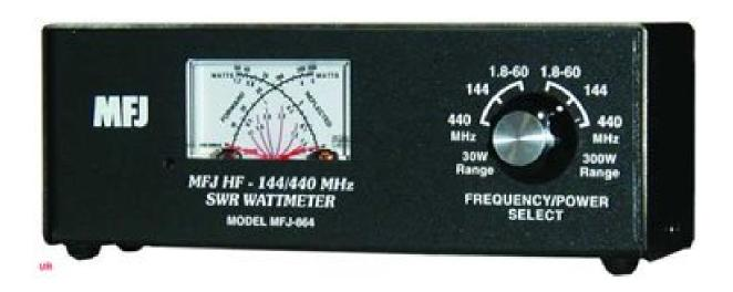
Note the use of the cross-needle meter to avoid the need to "cal" the measurement
