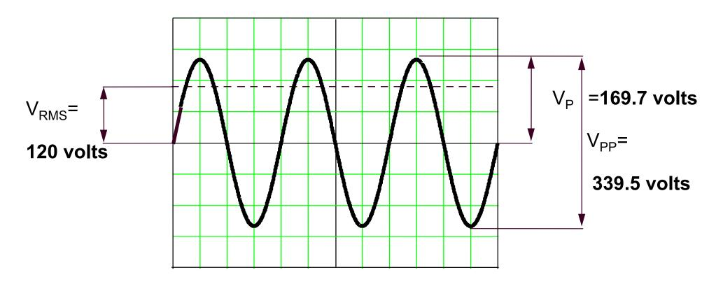
$V_{RMS} = 0.707 V_{P}$   $V_{P} = 1.414 V_{RMS}$
