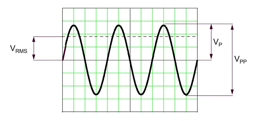
$V_{RMS} = 0.707 V_{P}$   $V_{P} = 1.414 V_{RMS}$
