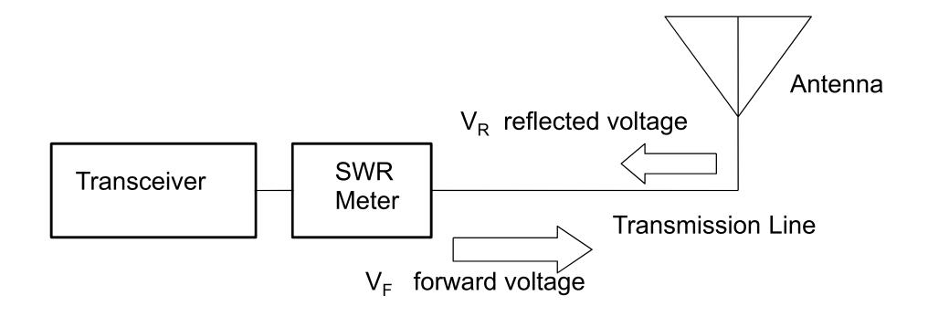
SWR meter is inserted into the transmission line, which usually requires an additional cable between transceiver and SWR meter.
