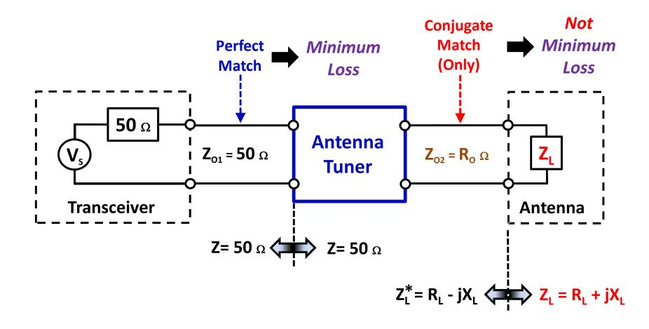
•Note: the "System" (not the antenna) has been "tuned" to resonance
