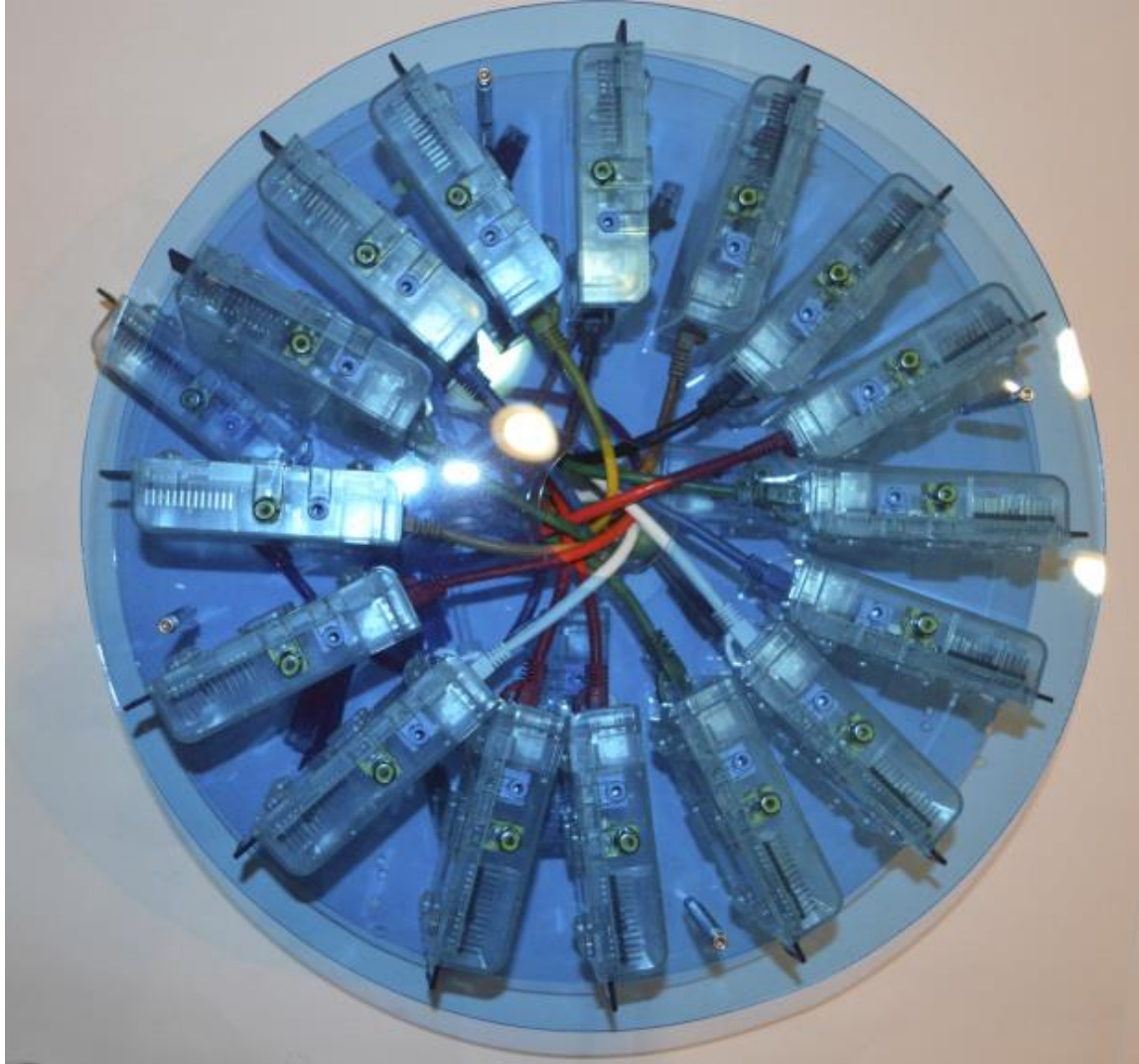
32 RPi low-cost “Supercomputer” Cluster
